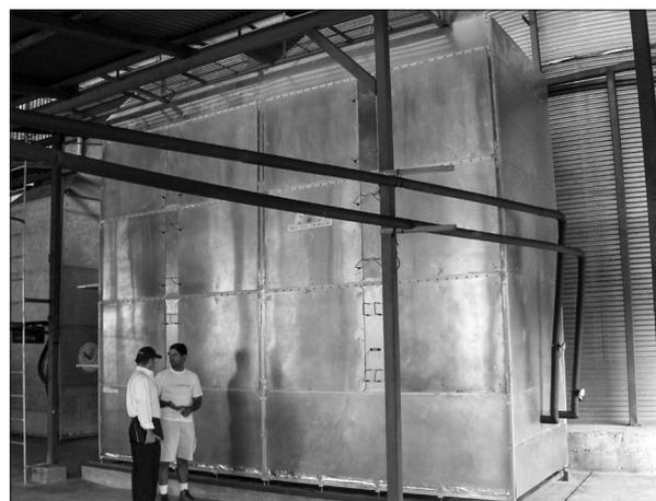
**Figure 1:** Industrial solar coffee dryers installed at the Montes de Oro Cooperative, Mirimar, Costa Rica. Each tower contains rotating trays on which coffee is placed for drying. Heat for drying is derived from exterior-mounted solar hot-water collectors as also for the gasification of coffee parchment
