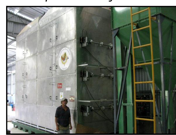
High-Efficiency Drying Chambers Manufactured in Massachusetts
